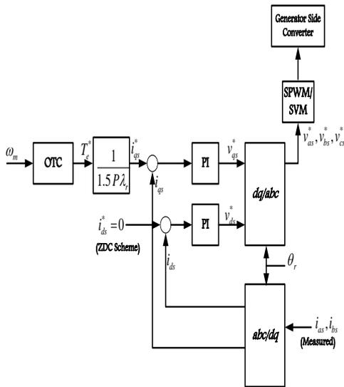
Figure 3. Generator side converter control scheme
