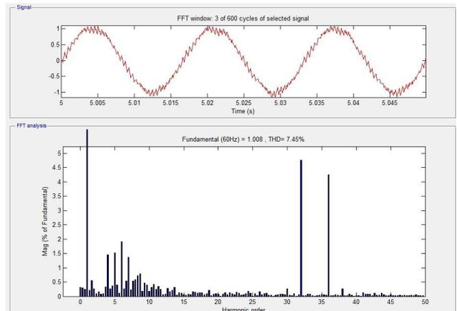
Figure 11. THD of Grid Current in PMSG based WECS
