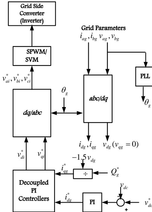
Figure 4. Grid side converter control scheme
