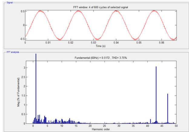
Figure 10. THD of Grid Current in DFIG based WECS
