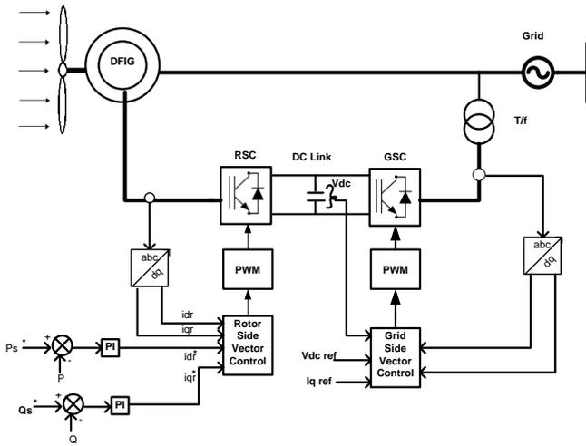
Figure 1. Block diagram of DFIG based Wind Energy Conversion System
