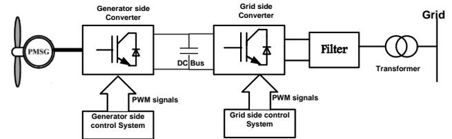
Figure 2. Block diagram of PMSG based Wind Energy Conversion System
