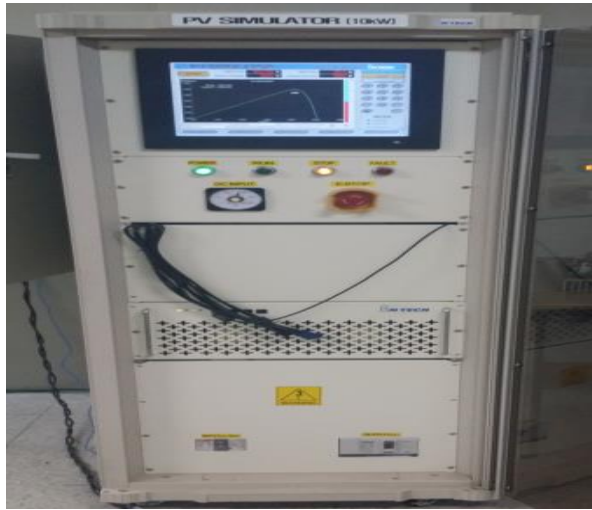
Figure 9. Test equipment used for electric power converter test.
