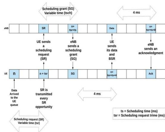
Figure 3. BSR mechanism
