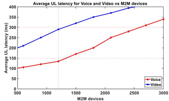
Figure 14. Average UL latency for Voice and Video versus number of M2M devices
