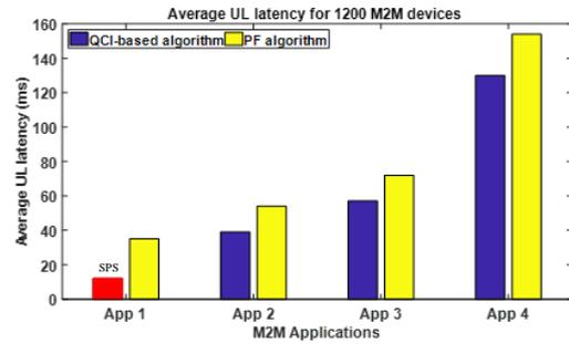
Figure 8. Comparison between QCI-based and SPS-based scheduling and PF
