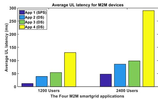
Figure 9. Average UL latency for each of the four M2M applications
