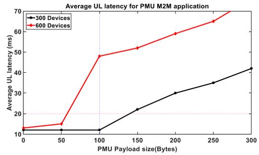
Figure 13. Average UL latency vs. PMU packet size
