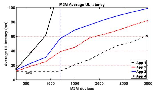
Figure 10. Average UL latency vs. number of M2M devices
