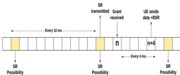
Figure 2. SR mechanism
