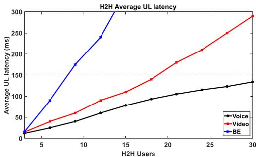
Figure 12. Average UL latency vs. number of H2H users for 1200 M2M devices
