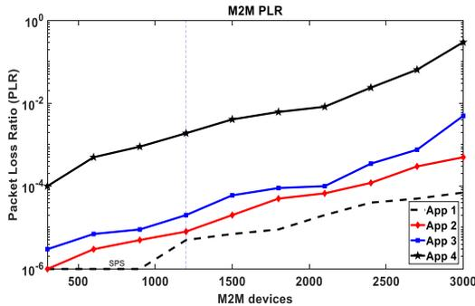
Figure 11. PLR vs. number of M2M devices
