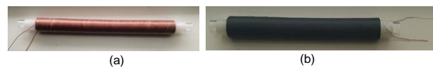
Figure 14. (a) AC Drive Coil Fig. 15(b) AC Drive coil with shrink wrap protection.
