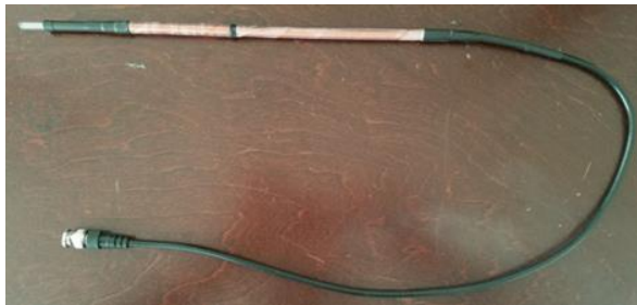
Figure 18. Detection and Cancellation Coil.
