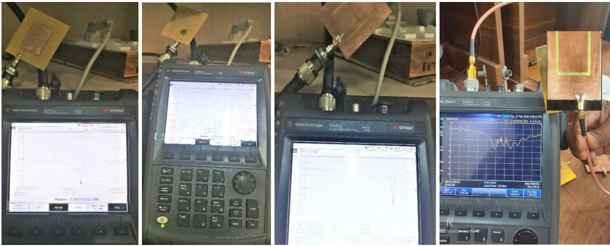
Figure 15. Experimental set up used for measurement of the radiation characteristics of the LSFMA without DGS and with O, H, and U shaped DGS.
