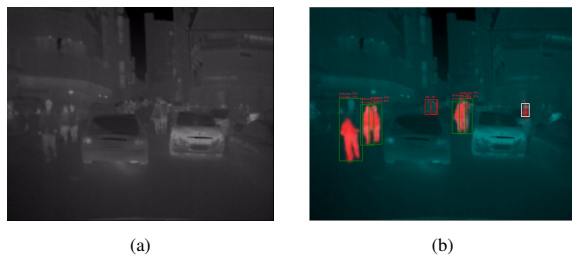
Figure 4. Example of TP, FP and FN for region-level F-measure calculation: (4a) original image, (4b) saliency output: TP(green BB), FP(white BB) and FN(red BB)
