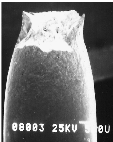
Figure 3 SEM photomicrograph of fractured specimen tested at -0.85 V (SCE).
